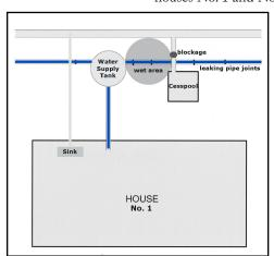
other by **stoneware** pipes six inches in diameter. A leaden pipe conveyed water from each tank to a pump situated in the back-kitchen. There is a cesspool behind each house, under the privy, and situated four feet from the water-tank. The ground was opened, and the drains examined under the superintendence of Mr. Grant, the Assistant-Surveyor, behind the houses No. 1 and No. 7. The cesspools at both these places were quite full,
